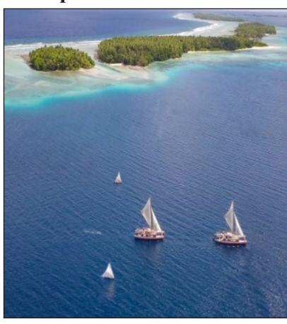
FSM is progressing well with its Sea Sustainable Transport proposal for the Green Climate Fund. The Vaka Motu (boat for the islands) – is a traditionally designed sailboat built with modern materials and propelled by fossil fuel-free technologies: solar and biofuel (coconut oil).
